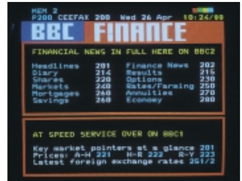
A Teletext page with the indication that it is a Fastext page – a small colour bar appears in the upper right-hand corner of the screen
